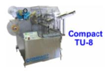
The standard machine consists of an infeed slide - adjustable by one screw knob for different size tubes. The infeed slide and pusher mechanism conceived by Compact is quite unique and while providing a large tolerance for setup - ensures zero rejects during the loading of the tube on the mandrels, even if the tubes have been previously damaged. The unique features of this machine will be forwarded to interested customers, please contact us for specific requirements.
